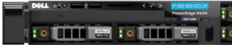
Figure 6. LCD control panel for 8-drive bay chassis
