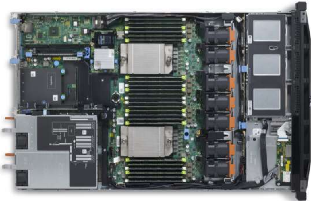
Figure 5. Eight-drive bay chassis internal view
